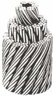
a. Multi-Strand Rope Construction
