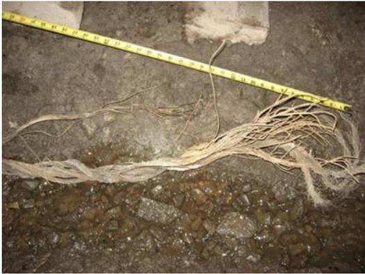
Failed end of the wire rope (car side) following the accident.
