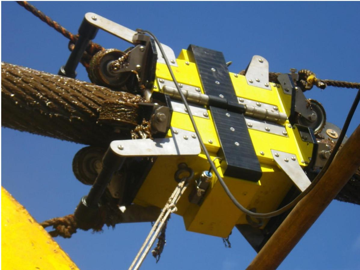
**Figure 2. [Magnetic Testing \(MRT\) of 160 mm diameter A&R Winch Rope](#)**
