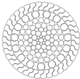
Typical 32 mm locked coil construction
