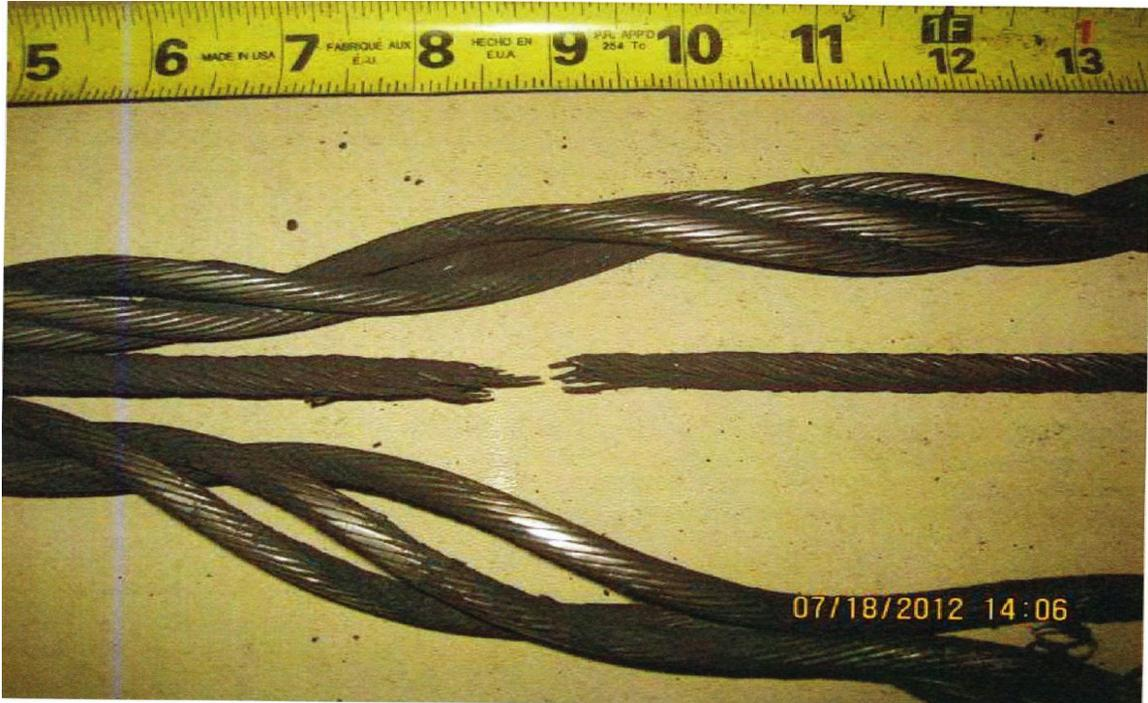
**Figure 7. 7/8 inch diameter, 6 x 25 FW RRL IWRC wire rope after disassembly**
