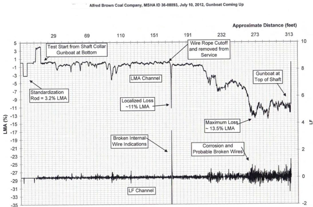
Figure 6. 7/8 inch diameter, 6 x 25 FW RRL IWRC wire rope MRT chart
