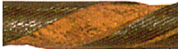
Corrosion in the first and second layer of the rope
