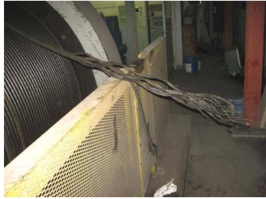
Failed end of wire rope (hoist drum side) following the accident.
