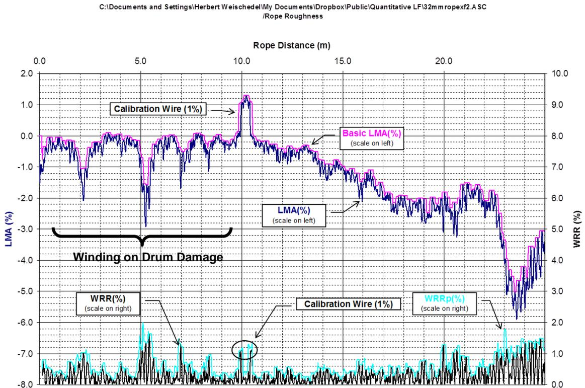
**Figure 5. 30 mm locked coil rope MRT NDE chart**
